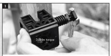
Place adapter on mounting structure. Engage  $\frac{1}{2}$ " wrench on top head and tighten at a slow and steady pace. The top head is designed to snap at the correct torque. Do not tighten further.
