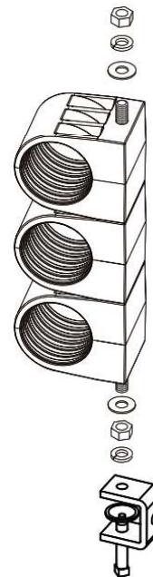
Hanger Clamp utilizing Triple Stack Hanger Kit CBAHXXTS8-Series
