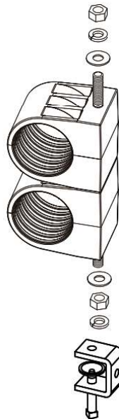
Hanger Clamp utilizing Double Stack Hanger Kit CBAHXXDS8-Series
